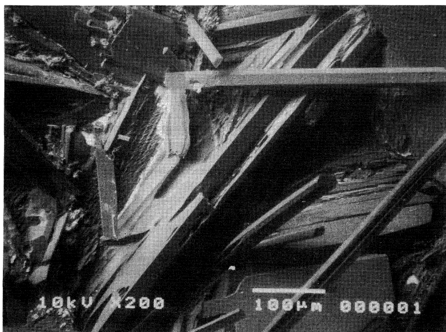
Fig. 1. SEM image of crystals of quinhydrone. Specimen produced from NaCl solution.
